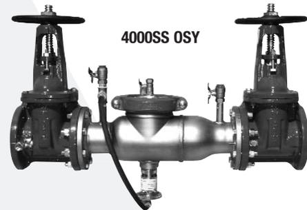
Series 4000SS Reduced Pressure Zone Assemblies are designed to provide protection of the potable water supply in accordance with national codes. This series can be used where approved by the local authority having jurisdiction on health hazard cross connections. Series 4000SS features short lay length, lightweight stainless steel body, corrosive resistant stainless steel relief valve, and patented cam-check assembly.
